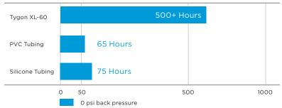
The performance of tubing in peristaltic pumping applications is affected by the conditions of use and equipment utilized, along with size and wall thickness of the tubing tested. The data above is presented for information only and should not be utilized for specification purposes.
